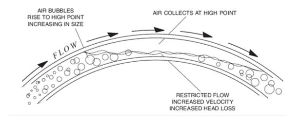
A float-actuated priming valve, installed in the suction side high points, is used with a vacuum priming system to establish pump prime, while keeping the liquid side of the process separate from the vacuum system. By allowing the continuous removal of air from the suction piping, it also helps ensure that pumps operate at peak design capacity without the possibility of becoming air bound or losing prime. Priming valves are a critical component of any vacuum priming system.
